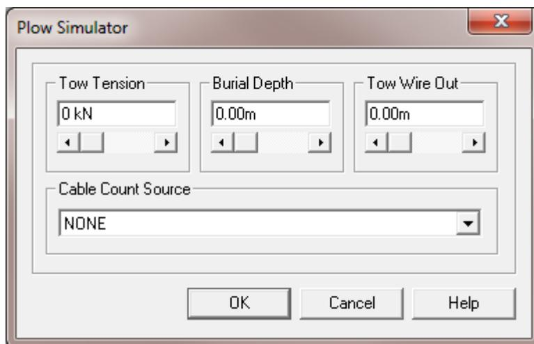
In the Tow Tension, Burial Depth and Tow Wire Out fields, you can either type in or use the scroll bar to enter values to be used by the simulated plow device. From the drop down list, select the Cable Count Source; typically this will be the Simulated Counter device.
